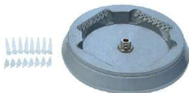
Angle Head 4 PCR strips of 96 wells
