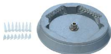
Angle Head 4 PCR strips of 96 wells
