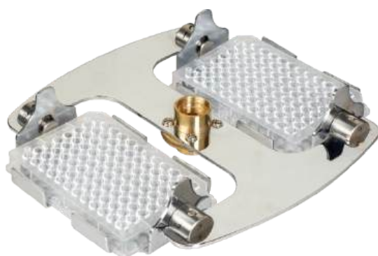
Swing out head 2 plates of 96 wells
