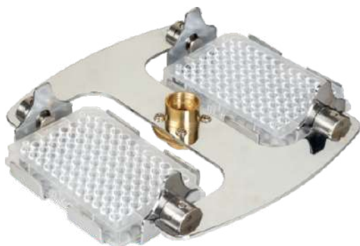
Swing out head 2 plates of 96 wells
